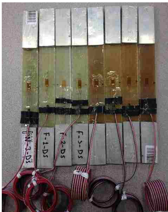
Figure 16. Color comparison between the control (left) and UV conditioned (right) specimens
