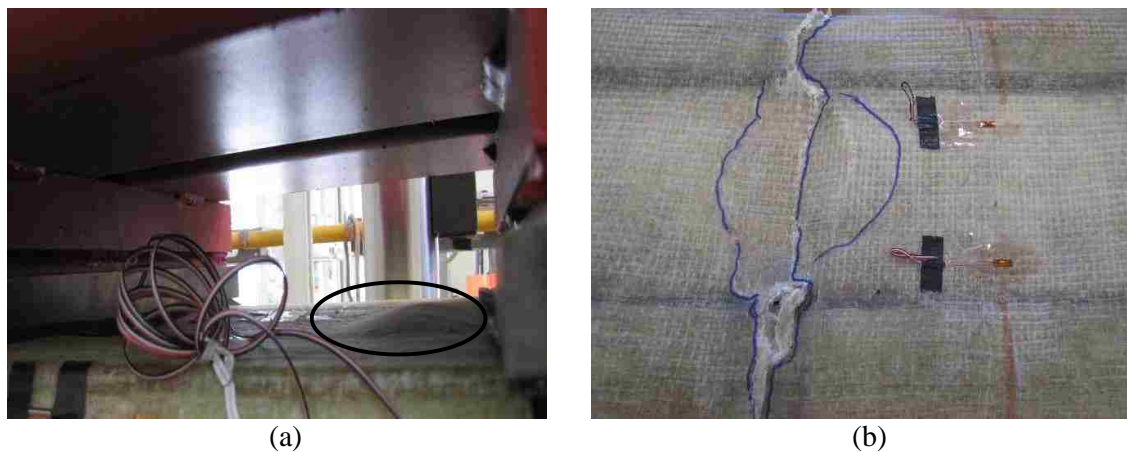
Figure 18. Failure modes: (a) initial failure due to outward compression facing wrinkling and (b) ultimate failure due to compression failure of the facesheet under loading points
