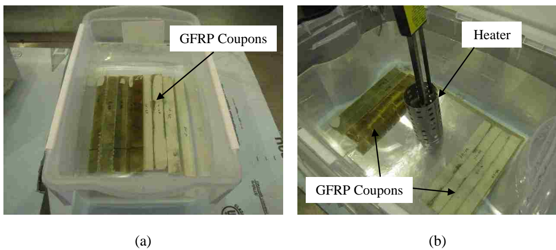
Figure 4. Deicing exposure: (a) coupon specimens at room temperature and (b) at elevated temperature
