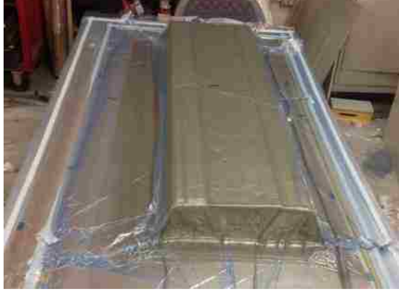
Figure 7. VARTM manufacturing process for mid-scale panels
