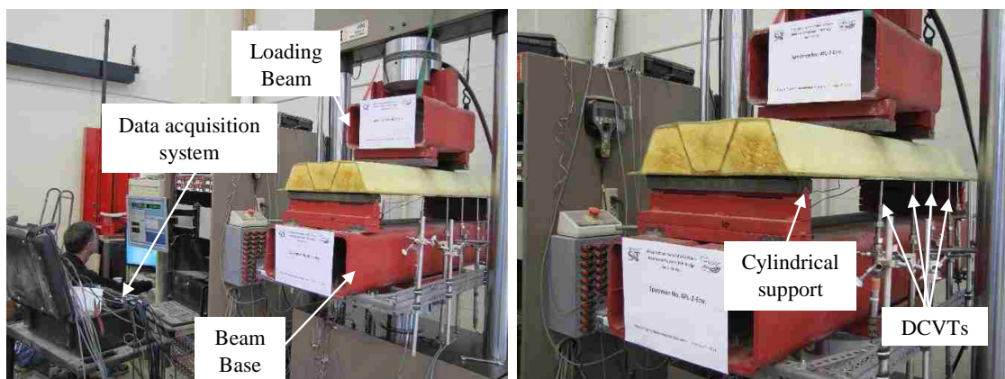
Figure 9. Four-point bending flexural test setup
