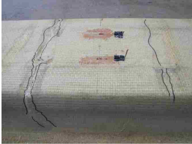
Figure 19. Compressive failure of the facesheet under loading points
