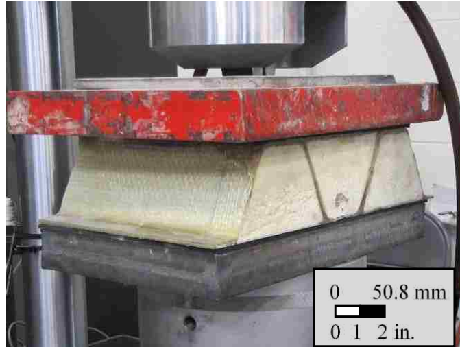
Figure 7. Crushing test setup
